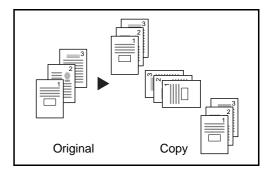
**NOTE:** To use the offset function, load the same sized paper with different orientation in the paper source other than the selected paper source.
