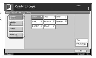
If you select [Size Entry], press [+] or [-] to specify *X* (horizontal) and *Y* (vertical) sizes. You can enter the size directly using the numeric keys after pressing [# Keys].
