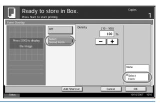
**NOTE:** You can change the form density setting through 10 levels from 10% to 100%. Press the [+] or [-] buttons in Density.
