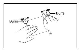
rough edges developed by a paper cutter on the back side. Remove any such rough edges by placing the Hagaki on a flat surface and rubbing the edges gently a few times with a ruler.
