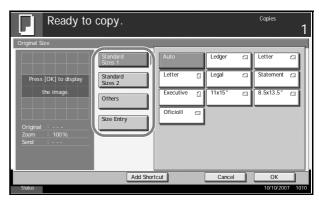
If [Size Entry] is selected, press [+] or [-] to specify the horizontal size (X) and the vertical size (Y). Press [# Keys] to enter the size directly using the numeric keys.
