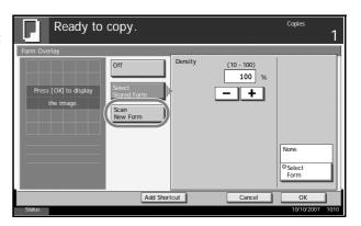
**NOTE:** Press [+] or [–] in [Density] to adjust the density of the form. Choose from ten levels in 10% increments.
